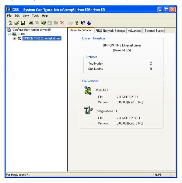
When the driver has been added to the relevant station then you are ready to proceed with setting up the FINS network parameters applicable to the PC. This is done by clicking the "FINS Network Setting" tab:
