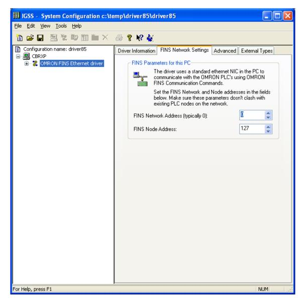
On the "FINS Network Setting" page you specify the FINS network parameters for the PC:
