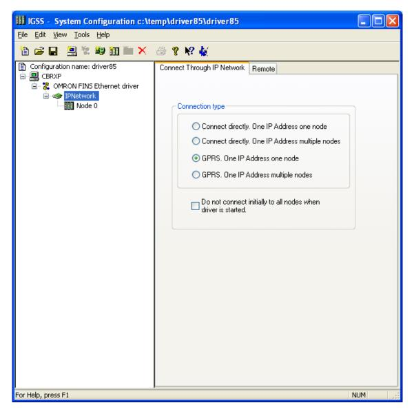
To enable this mode for the driver select the "GPRS. One IP Address one node" option as shown above.
