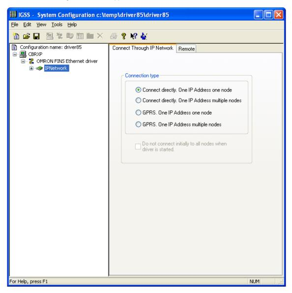
The Omron FINS Ethernet driver is designed to use one IP address for each node and thus you should select one of the options:
