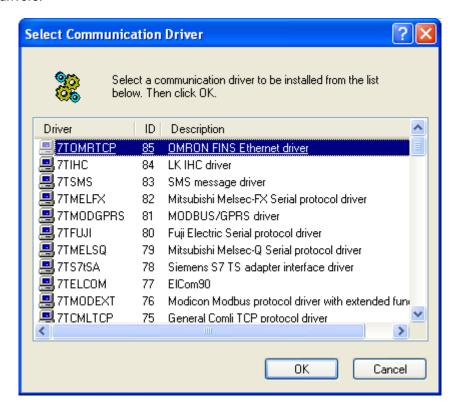
If the driver is present then you can proceed to the next section: "Configuring the Driver", otherwise install the driver using the manual installation procedure described below.
