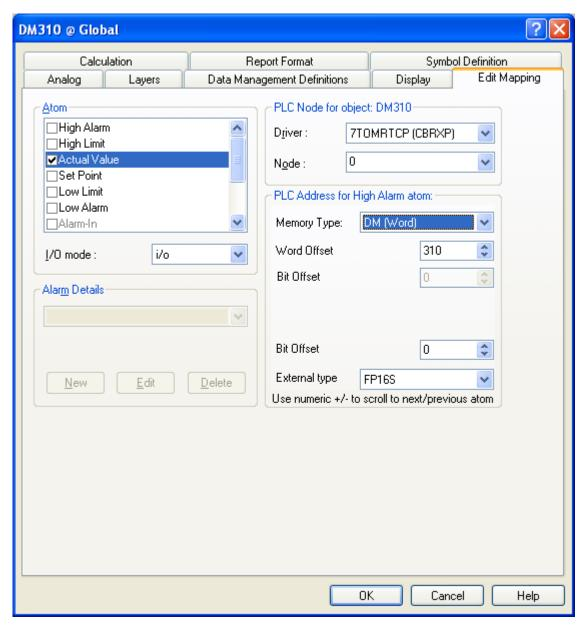
Now select the desired PLC node number and continue by setting be desired Device. Then specify the number (register number within the device type). Note that the corresponding Mnemonic is displayed and updated as you select the appropriate parameters. This is a help to make sure you always bind to the correct process variable.
