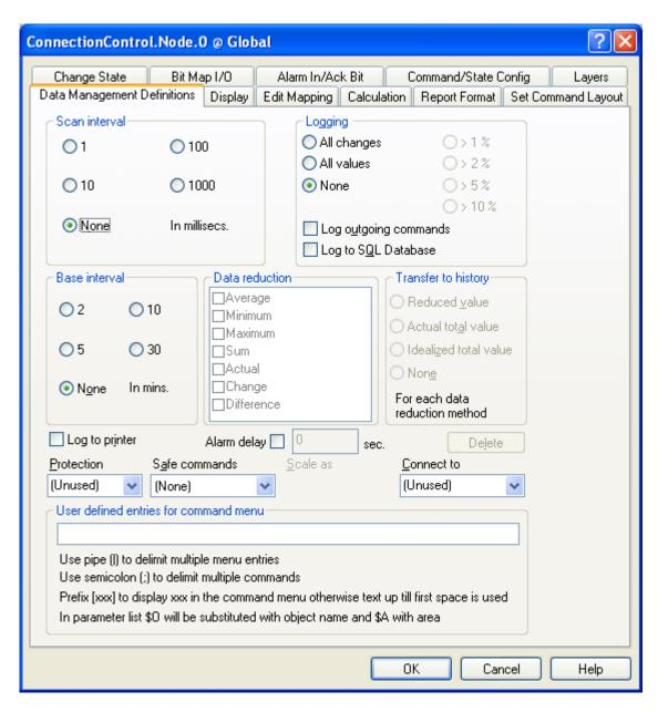
And bind both the Command- and the State atom to "Historical Data (Word)" and Word Offset 0 (this corresponds to parameters 512 and 0 we just set up in the "Connection Misc." pane for the driver).
